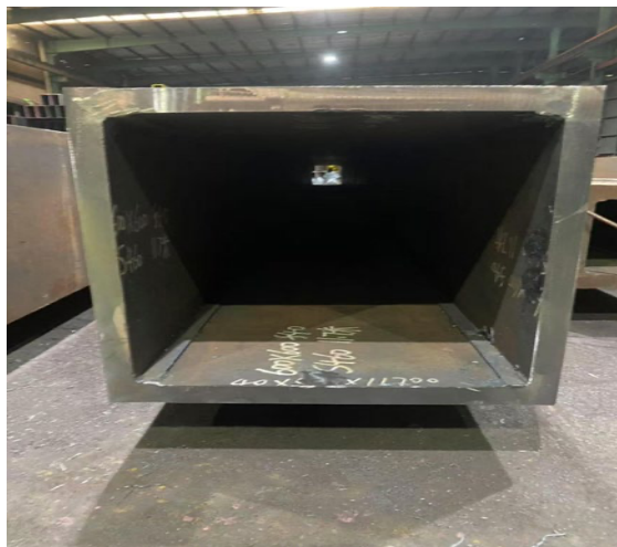
Figure 2 Structural steel built ups
